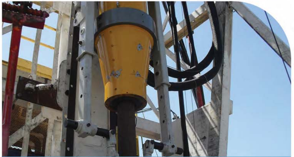
Casing Running Tool Testing in Houma
