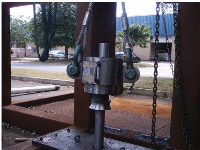
CableGrab umbilical and cable removal tool gets a firm grip during testing.
