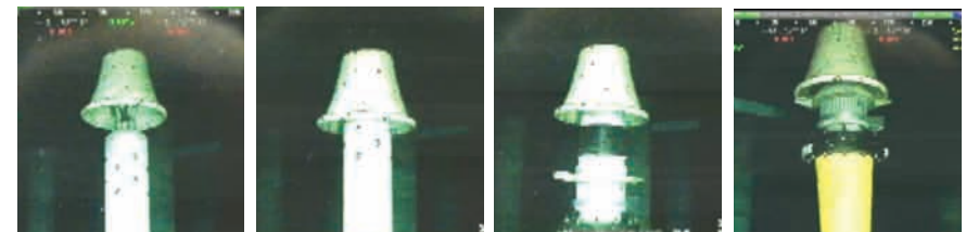
Subsea connection without diver intervention
