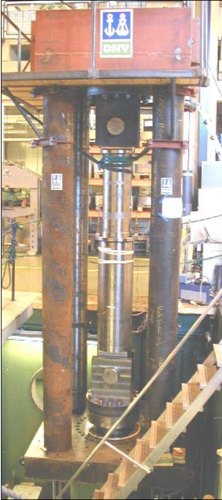
Figure 22 Anchor connector installed in test rig.
