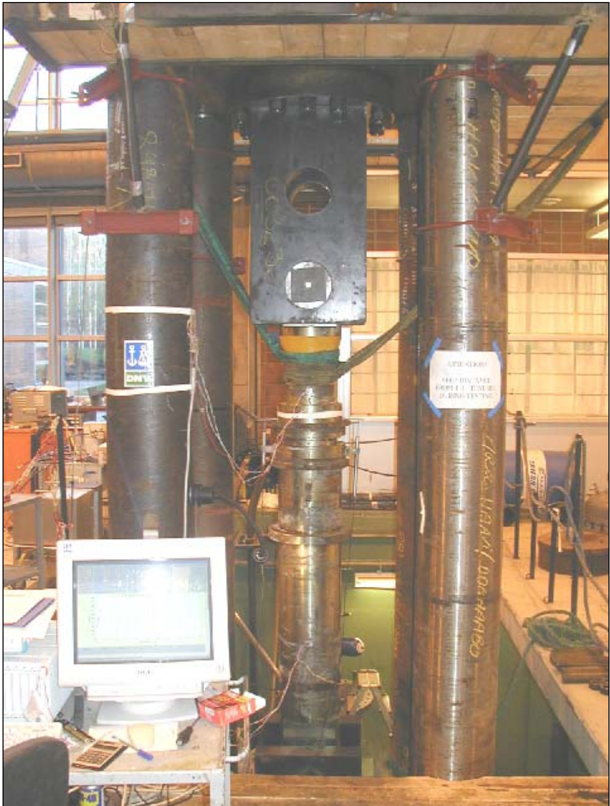
Figure 27 Anchor connector installed in test rig.
