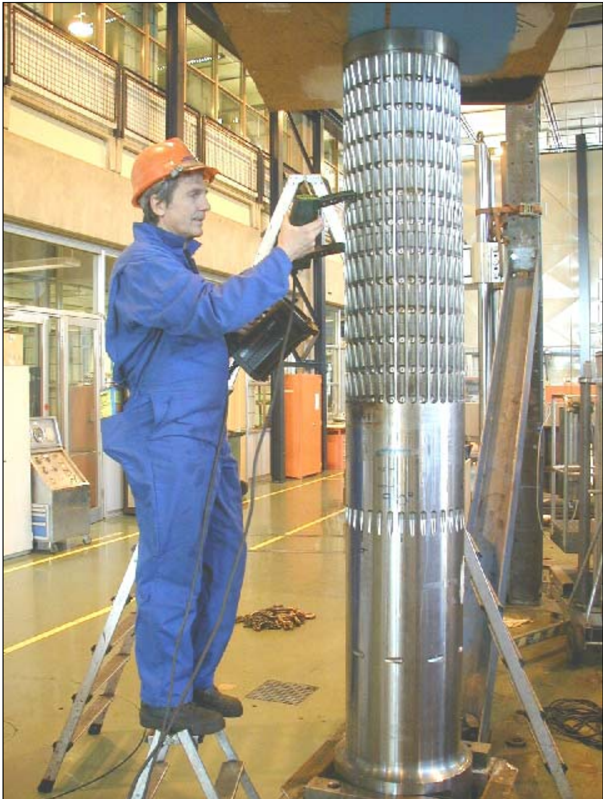
Figure 20 Magnetic particle inspection (MPI) after testing.
