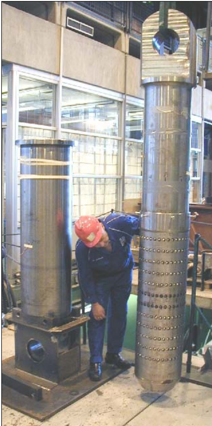
Figure 23 Anchor connector disassembled after testing.
