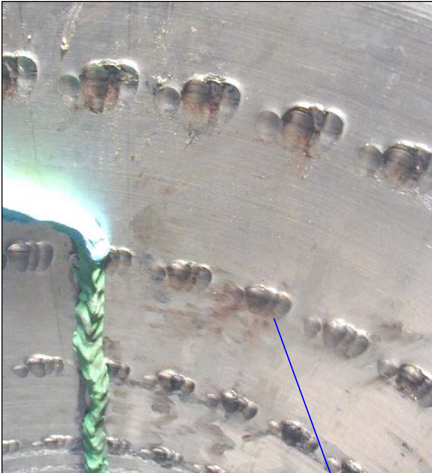
Figure 25 Close-up of indents inside of receptacle after testing.
