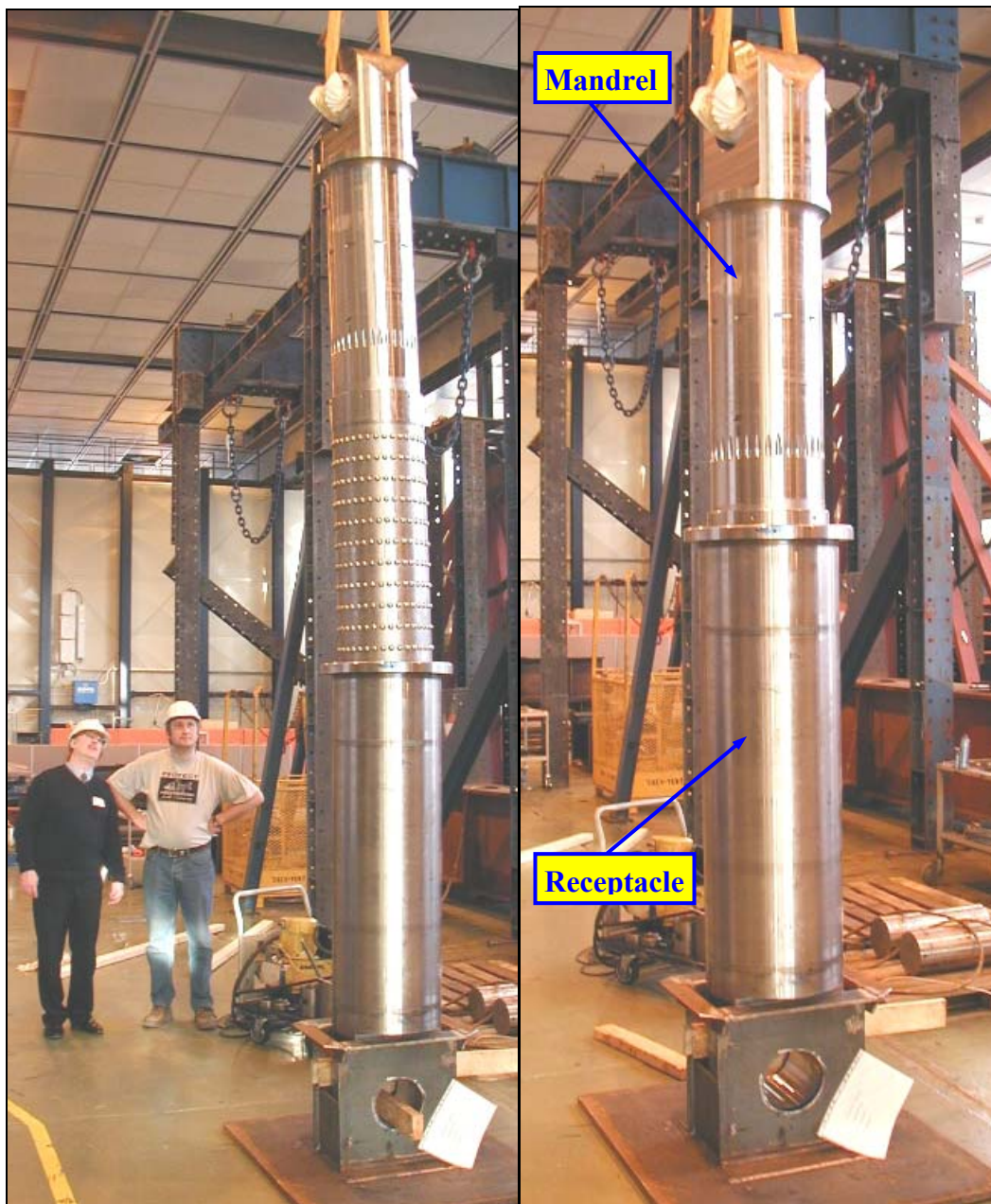
Figure 3 To the left: 1500t MBL Ballgrab Anchor Connector being connected. To the right: 1500t MBL Ballgrab Anchor Connector after connection.
