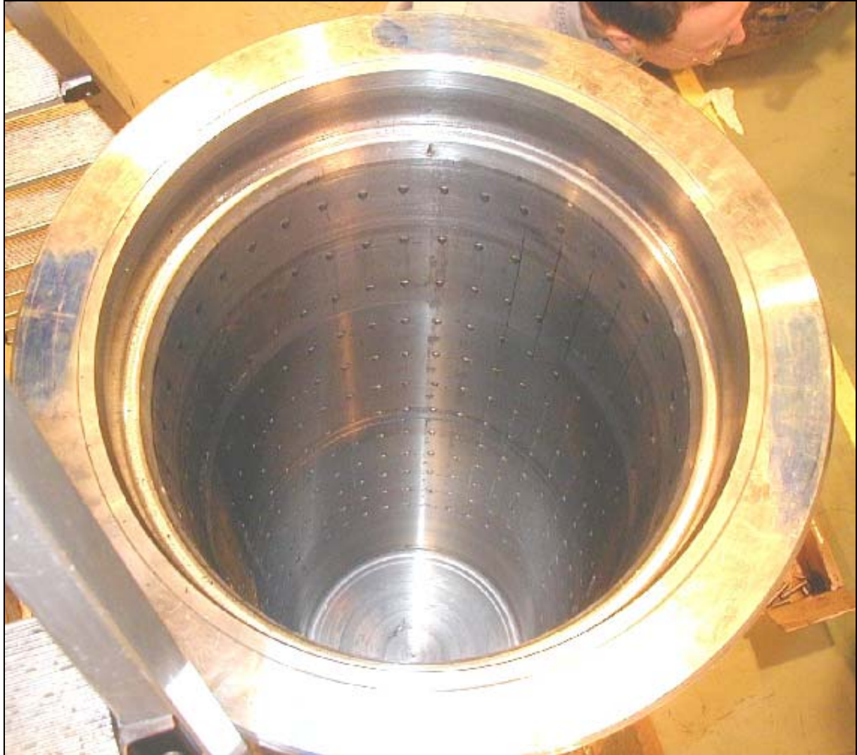
Figure 11 Indents in the receptacle after functionality test.
