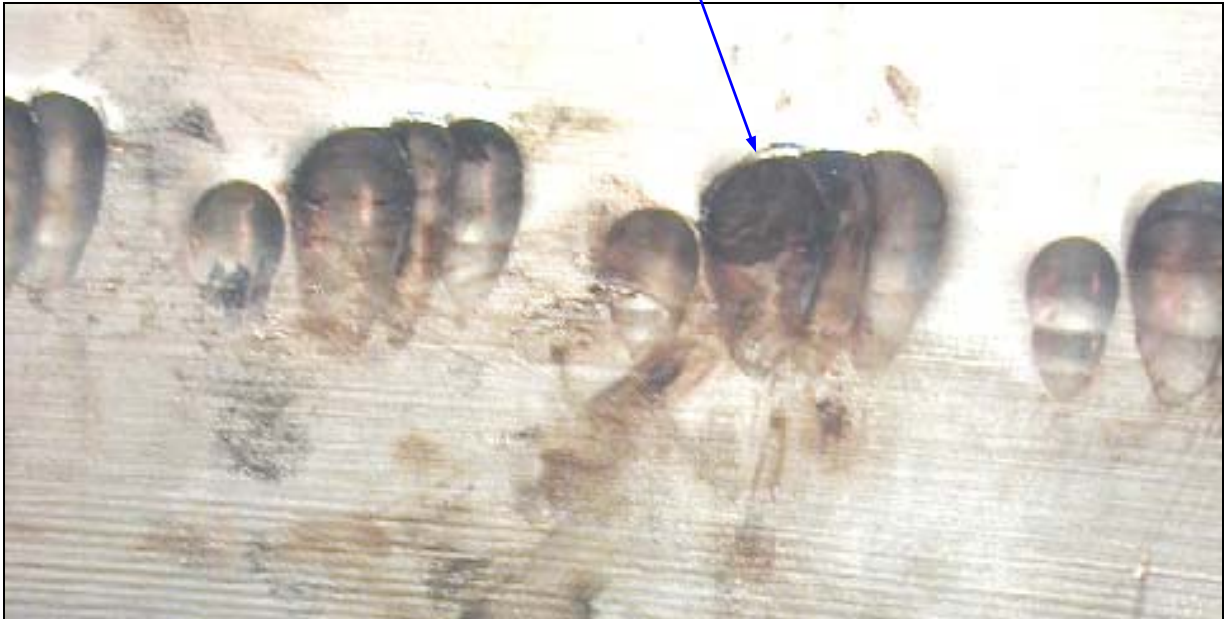
Figure 26 Close-up of indents inside of receptacle after testing.
