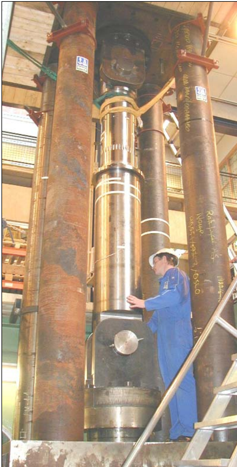
Figure 14 Anchor connector installed in test rig (with two rows of balls).
