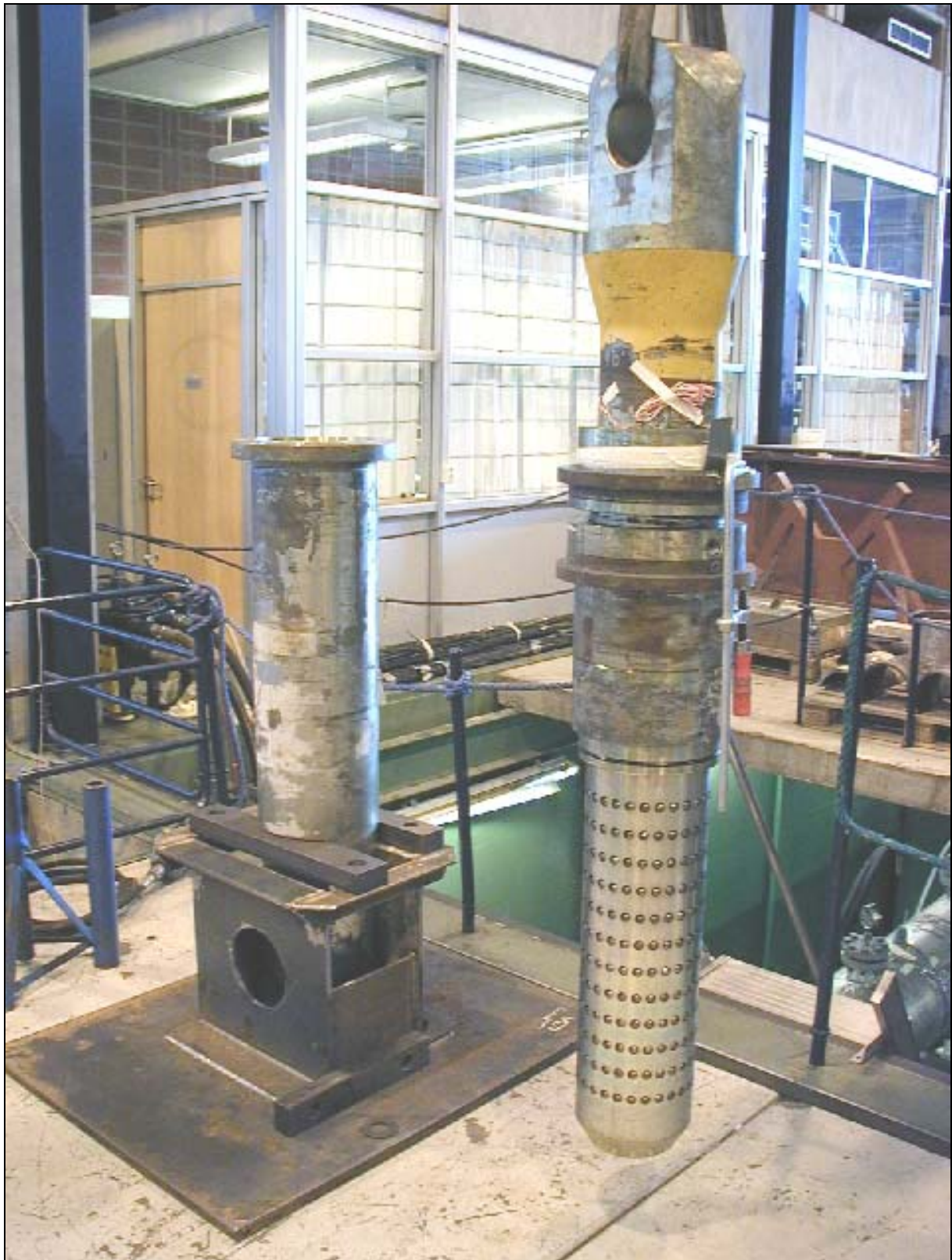
Figure 28 Anchor connector disassembled after testing.
