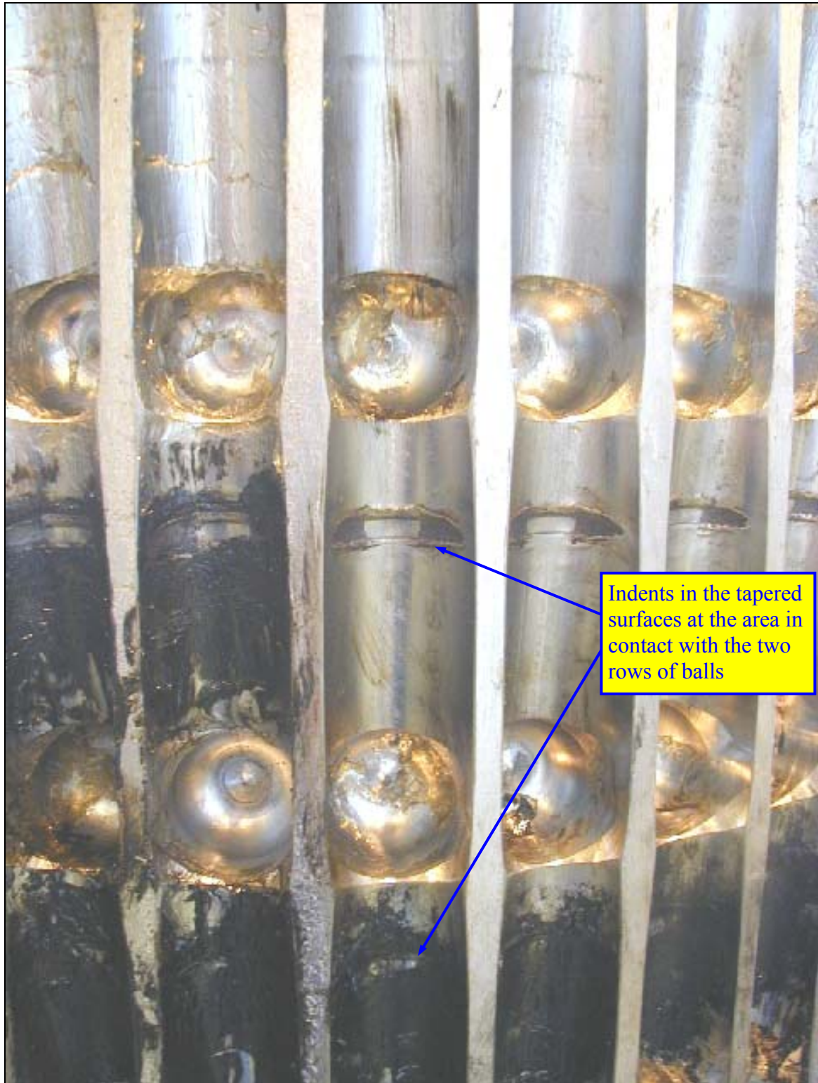
Figure 17 Close-up of tapered surfaces on mandrel after testing.
