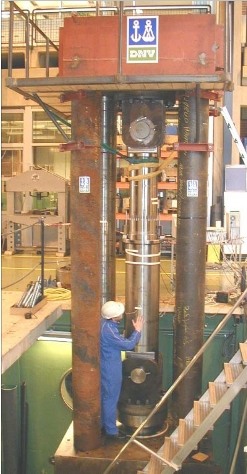
Figure 6 Fatigue testing of 1500t MBL Ballgrab Anchor Connector.
