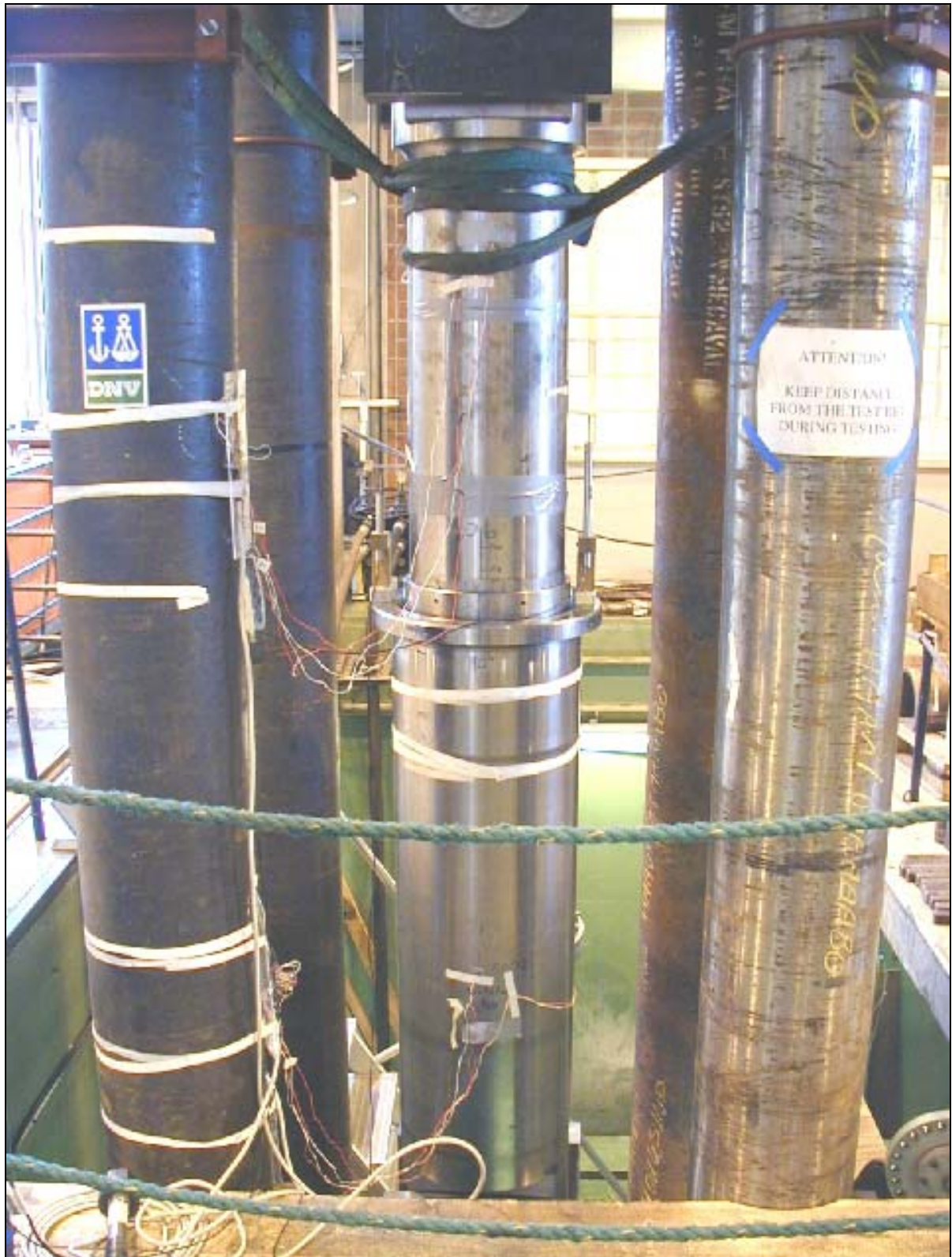
Figure 21 Anchor connector installed in test rig.
